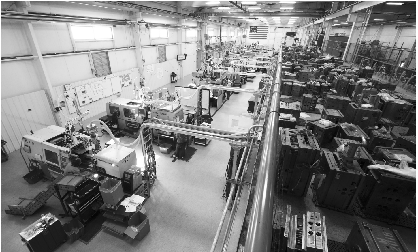
Storing tools and dies adjacent to presses on the mezzanine level of the plant saves operators setup time.
