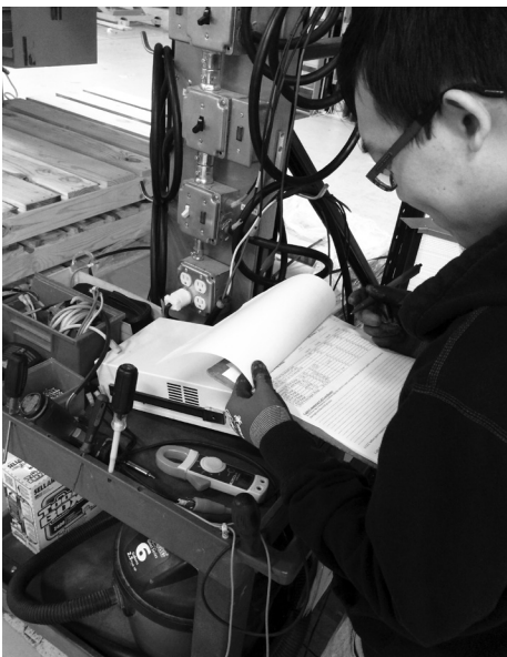
Technicians perform and record full-function testing of each unit they assemble, a standard practice at RenewAire.
